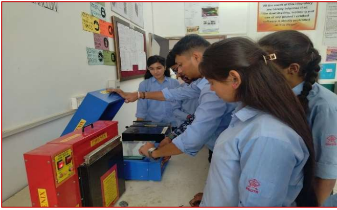
Exposing to UV light through Negative Image
